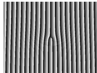
Fig. 2. Forked hologram for producing doughnut modes via SLM.
