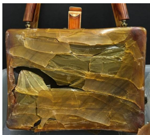
Fig. 1. V&A collection. Degradation of a plastic handbag
